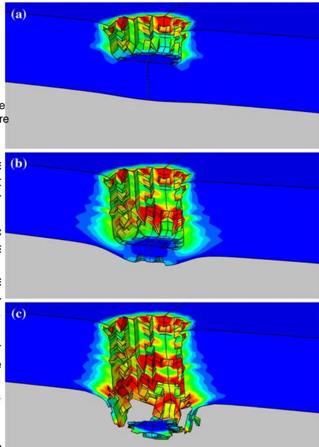
Fig. 9 The spatial distribution of deformation and damage within the laminate as predicted by the laminate-scale material model at post-impact times of: a 15  $\mu$ s, b 30  $\mu$ s and c 45  $\mu$ s. The initial FSP velocity = 300 m/s. Maximum principle strain range (0.05, 0.5)
