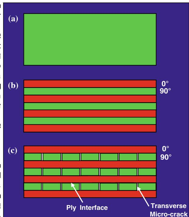
Fig. 1 Schematic representation of the composite laminate as represented by the laminate-scale material model; the classical meso-scale model, and the fracture-mechanics enriched meso-scale model. The one developed over the last 20 years by Ladeveze and co-workers [1, 2] appears to be the most advanced. Consequently, the first objective in the present work is to provide a critical assessment of this model (the Ladeveze meso-scale model, in the following).
