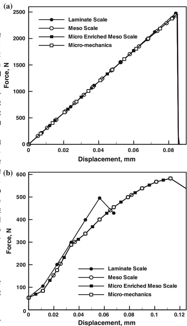
Fig. 3 Variation of the uni-axial force with the uni-axial displacement in the cases of (a) in-plane tension; and (b) in-plane compression of a prototypical  $[0/90_2/0]_s$  carbon-fiber reinforced epoxy matrix composites
