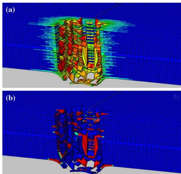
Fig. 16 The spatial distribution of damage variables at 30 FSP post-impact time within the laminate as predicted by the micro-mechanics-based material model: a) d'Nrange (0.005, 0.05) and b) d'Nrange (0.025, 0.25)
