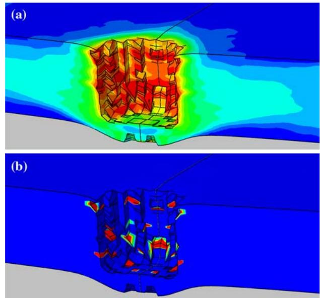
Fig. 13 The spatial distribution of damage variables at 30 FSP post-impact time within the laminate as predicted by the laminate-based material model: a  $d_f$  range (0.005, 0.05) and b  $d_f$  range (0.025, 0.25)
