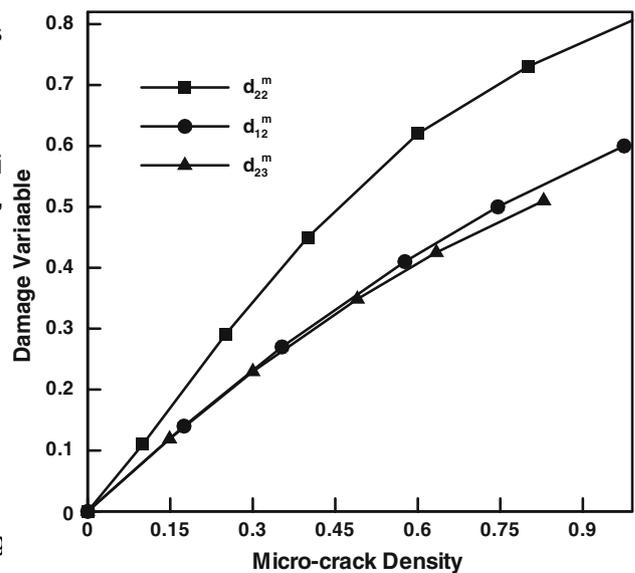
Fig. 2 Functional relations between the three damage variables associated with transverse micro-cracking with the micro-crack density parameter  $\rho$ . The three damage parameters, respectively, degrade the transverse Young's modulus, the transverse shear modulus associated with shear along the fibers, and the transverse shear modulus associated with shear in the through-the-thickness direction
