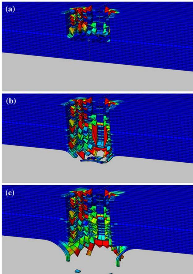
Fig. 12 The spatial distribution of deformation and damage within the laminate as predicted by the micro-mechanics-based model at post-impact times of a 15  $\mu$ s, b 30  $\mu$ s and c 45  $\mu$ s. The initial FSP velocity = 300 m/s. Maximum principle strain range (0.05, 0.5)
