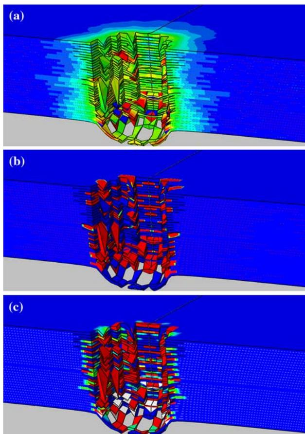
Fig. 15 The spatial distribution of damage variables at 30 FSP post-impact time within the laminate as predicted by the fracture-mechanics enriched meso-scale material model: a) d'Nrange (0.005, 0.05); b) d'Nrange (0.025, 0.25); and c) rho'Nrange (0.001, 0.02)
