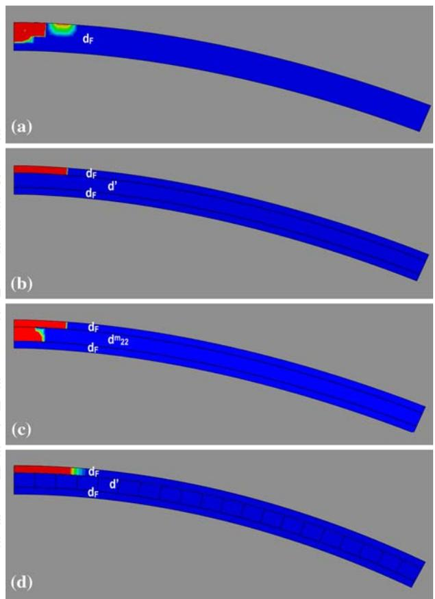
Fig. 7 Spatial distribution of the variables quantifying damage which leads to initiation of failure within the composite laminates: a the laminate-scale model; b the classical meso-scale model; c the fracture-mechanics enriched meso-scale model; d the micro-mechanics-based model. Damage variable range: (0.001, 0.005); Bending angle: 0.02
