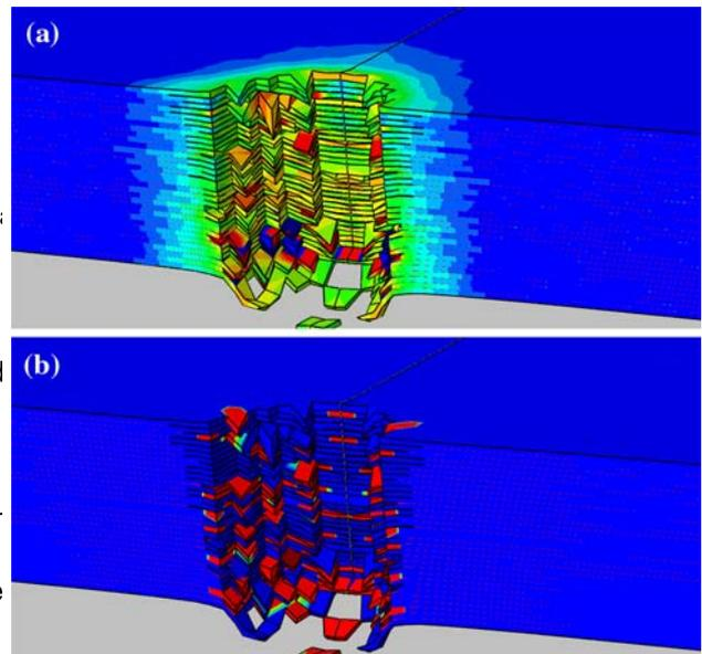
Fig. 14 The spatial distribution of damage variables at 30 FSP post-impact time within the laminate as predicted by the meso-scale material model: a  $d_f$  range (0.005, 0.05) and b  $d_f$  range (0.025, 0.25)
