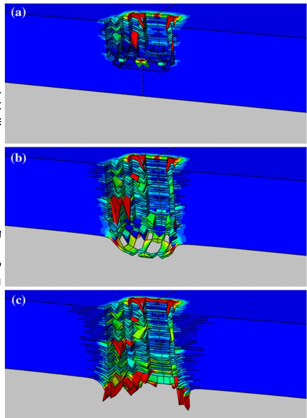
Fig. 11 The spatial distribution of deformation and damage within the laminate as predicted by the fracture-mechanics enriched meso-scale model at post-impact times of a) 15  $\mu$ s, b) 30  $\mu$ s and c) 45  $\mu$ s. The initial FSP velocity = 300 m/s. Maximum principle strain range (0.05, 0.5)
