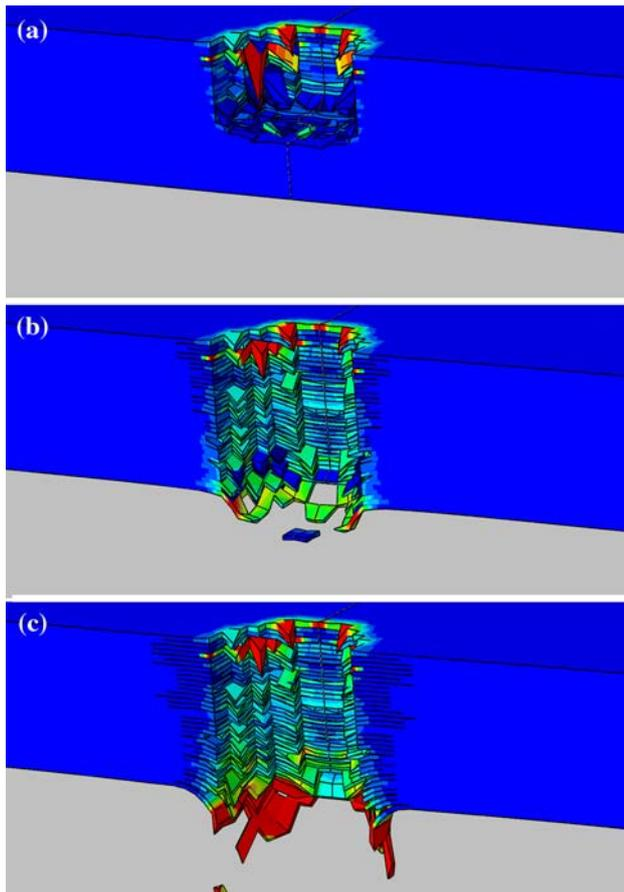
Fig. 10 The spatial distribution of deformation and damage within the laminate as predicted by the classical meso-scale material model at post-impact times of a) 15  $\mu$ s, b) 30  $\mu$ s and c) 45  $\mu$ s. The initial FSP velocity = 300 m/s. Maximum principle strain range (0.05, 0.5)
