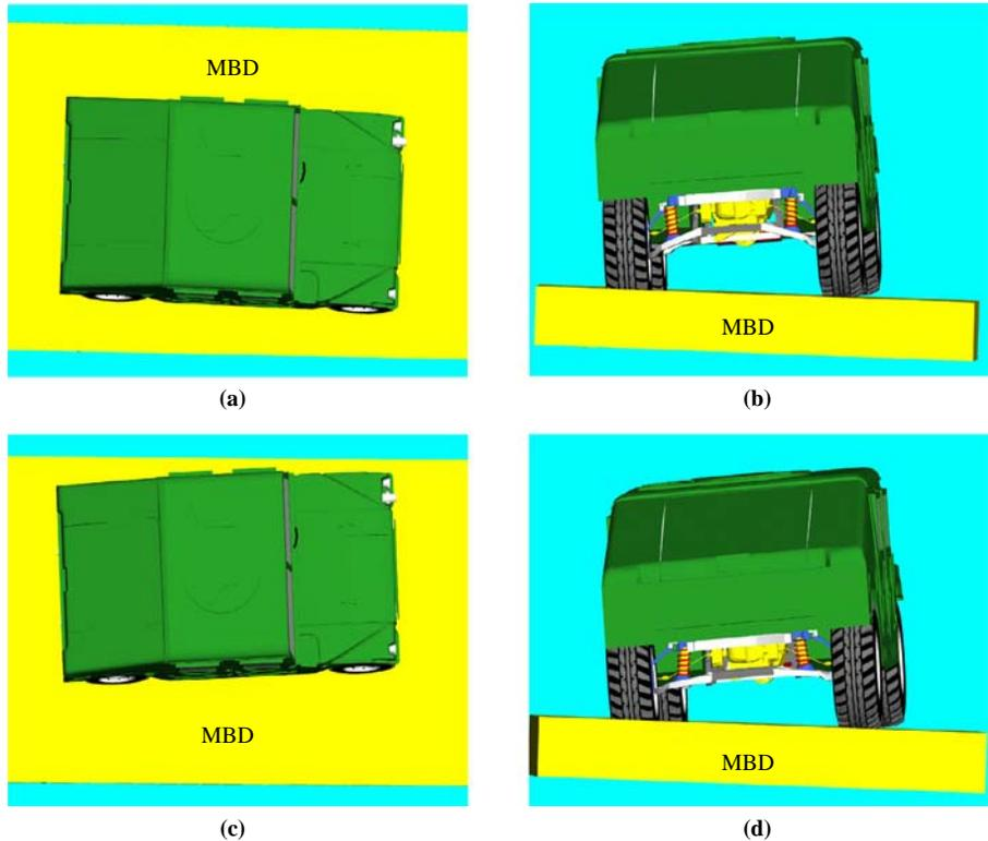
**Figure 9.** Qualitative evidence for the up-armor configuration increased rollover propensity in the HMMWV during a downhill braking maneuver obtained using MBDA analysis
