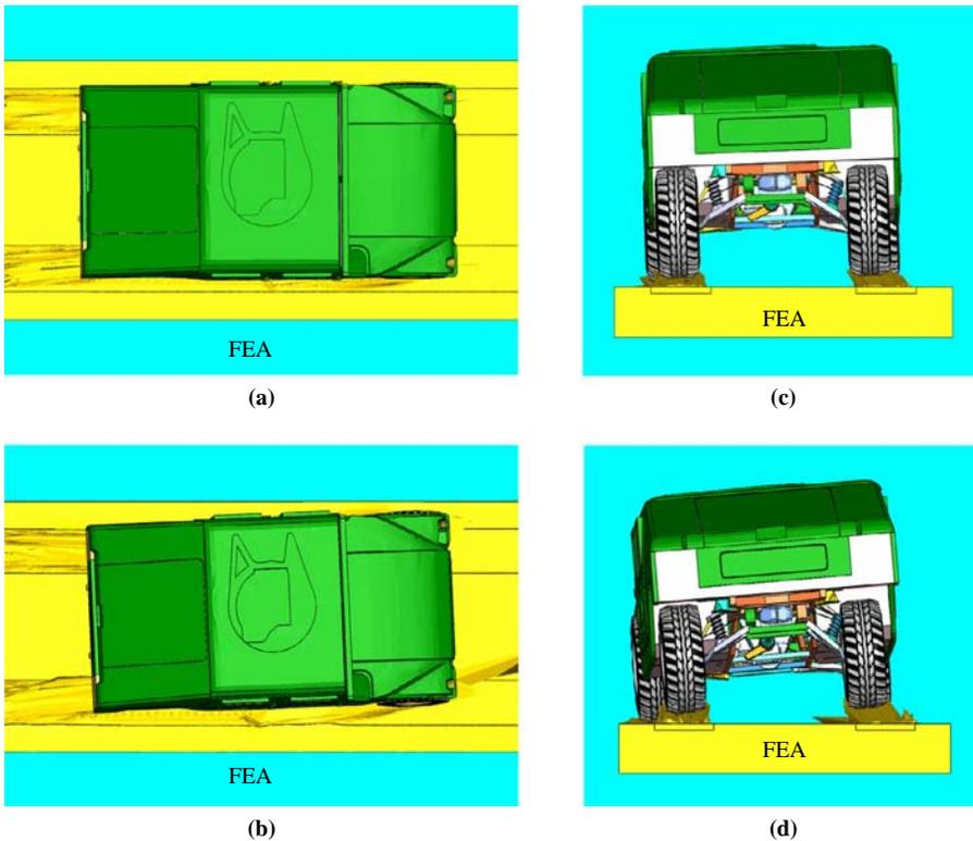
**Notes:** (a) and (c) Standard vehicle configuration; (b) and (d) up-armored configuration; (a) and (b) top views; and (c) and (d) rear views; pre-braking velocity = 27 km/h; please see text for details
