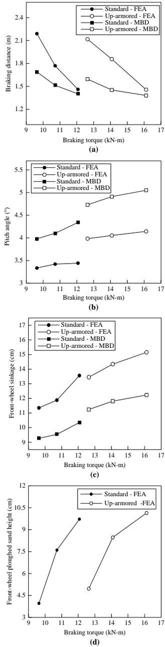
**Figure 6.** The effect of HMMWV up-armor and the average braking torque on the: (a) braking distance; (b) pitch angle; (c) front-wheel sinkage; and (d) maximum height of the front-wheel ploughed sand, for the straight-line flatland braking case
